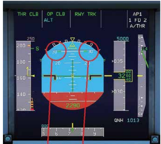
Pitch attitude protection nose up limit 30°
