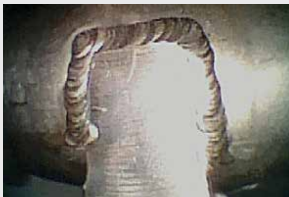
Using a borescope to inspect the welds of the engine nacelle anti-ice system. (Photo: Hawkeye videoscope.)
